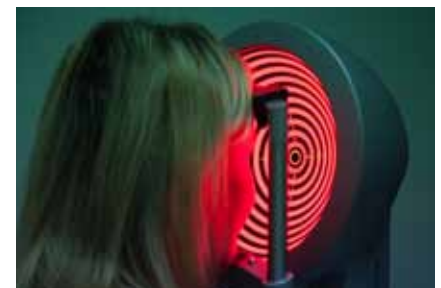
Figure 3. The WaveLight Topolyzer is a placido topographer that sends data to the excimer laser for topographic-guide treatment.
